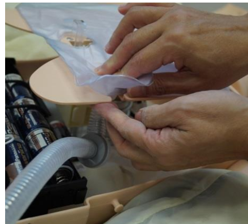
Step 14: Attach the disposable airway and secure it to the inner chest cover
